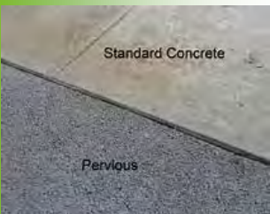
Pervious Concrete vs. Standard Concrete
